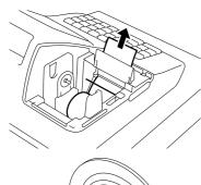
If the printer is used for Receipt, cut the paper roll as shown in the figure. Then hold down the **[FEED]** key to advance the remaining paper end.
